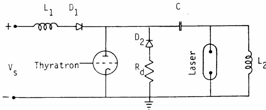
*Figure 11.* Schematic diagram of resonant charging circuit which permits the capacitor C to be charged to twice the power supply voltage (or more, depending on matching between discharge circuit and plasma tube).
