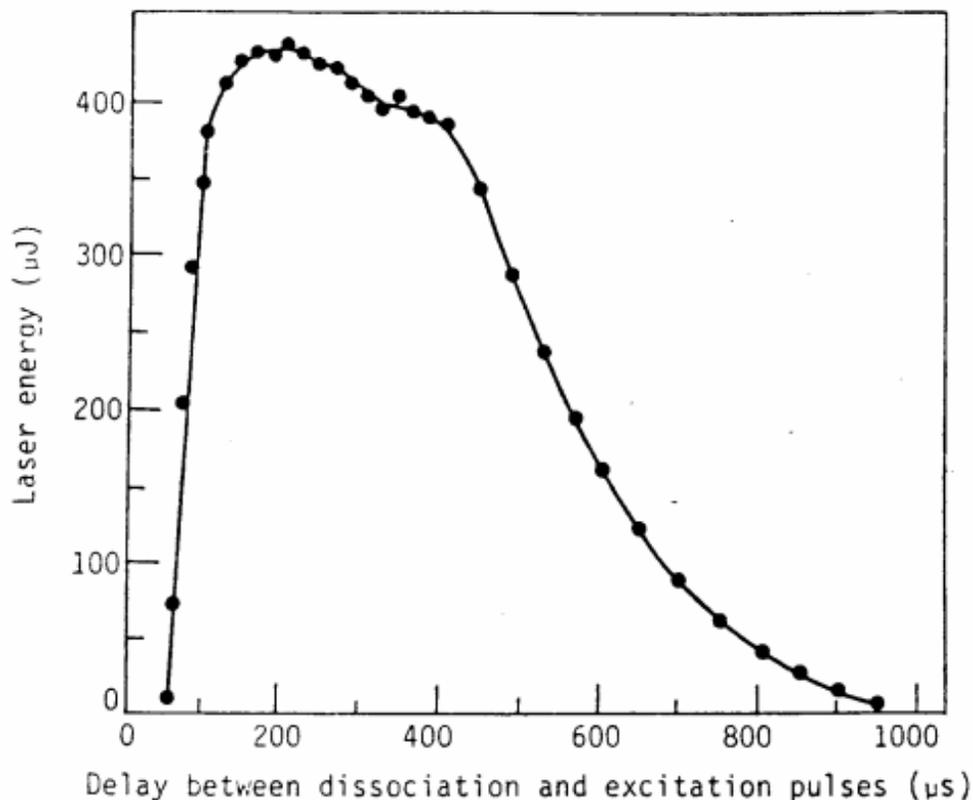
*Figure 4.* Dependence of laser output on delay between dissociation and excitation pulses. Tube length 22 cm, diameter 25 mm; Temperature: 430°C; He pressure: 4 torr; Dissociation energy: 2.4 J; Excitation energy: 2 J.
