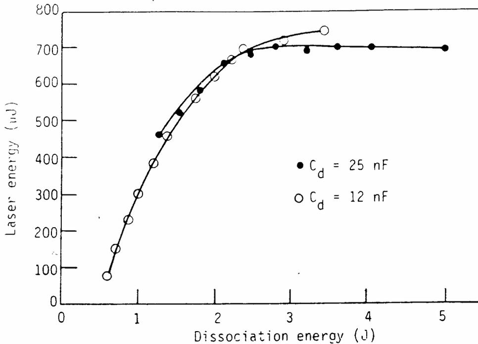
Figure 8. Laser output energy as a function of dissociation energy for two different dissociation capacitors. Tube length: 22 cm, diameter 30 mm; Temperature: 430°C; He pressure: 4 torr; Delay: 300  $\mu$ s; Excitation energy: 2 J.
