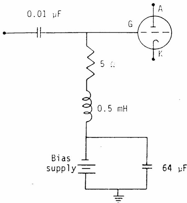
Figure 12. Grid circuit designed to minimize recovery impedance.
