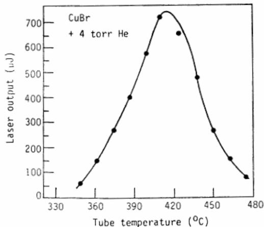
Figure 2. Dependence of laser output on tube temperature.
