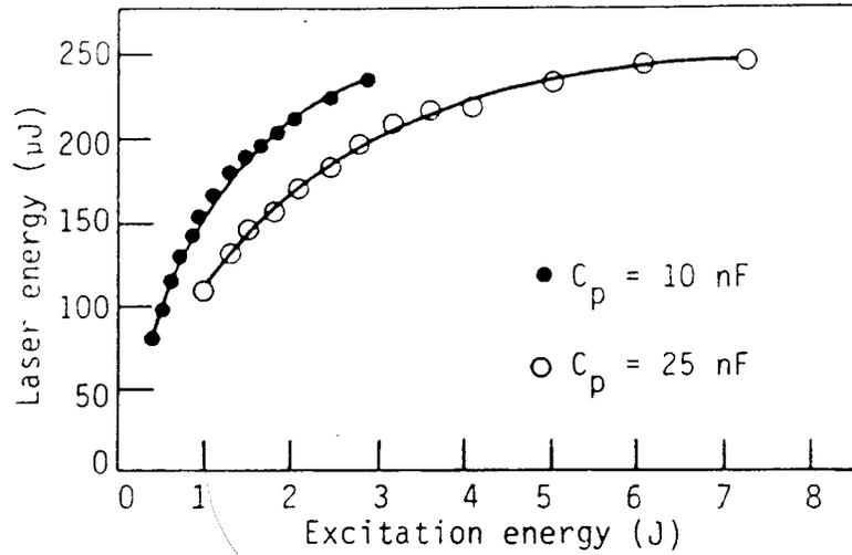
Figure 7. Laser output energy as a function of excitation energy for two different excitation capacitors. Tube length 22 cm, diameter 19.5 mm; Temperature: 430°C; He pressure: 3 torr; Delay: 140μs; Dissociation energy: 720 mJ.
