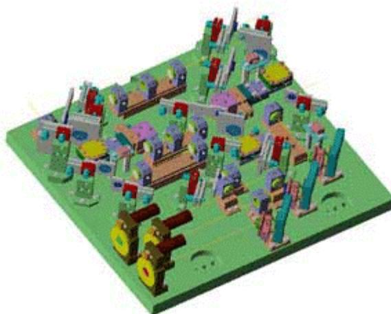
*Fig. 10 Nonlinear frequency conversion unit with dimensions of 370 x 340 mm<sup>2</sup>.*
